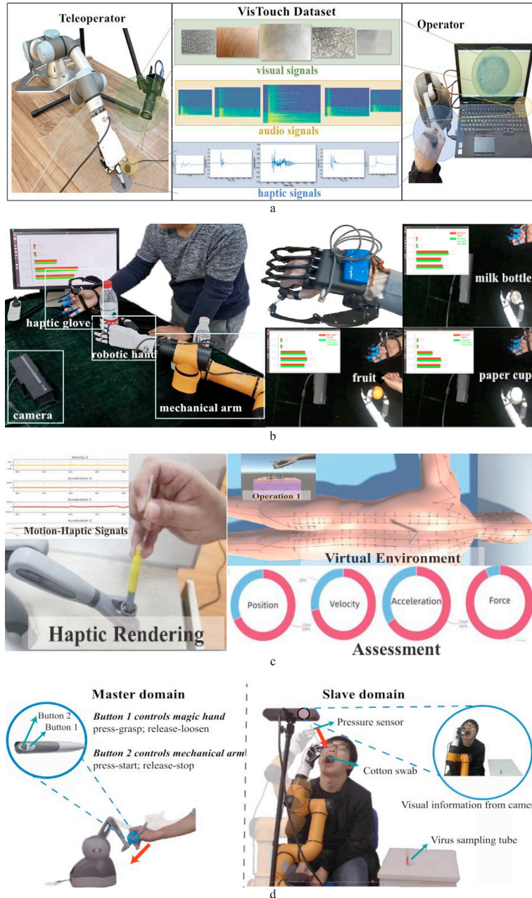
Fig. 6. Illustrations of the developed prototype systems: a Large-scale cross-modal communication-related dataset; b Visual-haptic human-machine interactive system; c Virtual interactive acupuncture skill training application [60]; d Remote throat swab sampling platform [64].
